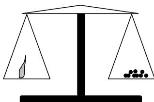
We can estimate the mass of light objects by picking them up. This is called hefting. We compare the feel with the feel of objects whose mass we know, for example with a litre of milk which has a mass of 1 kg or with a bean which has a mass of about a gram.
