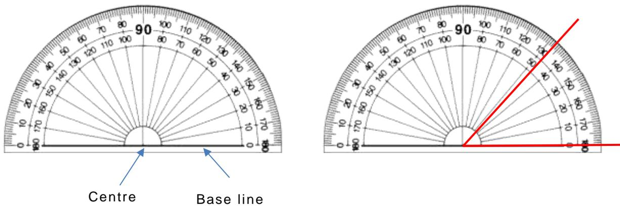
Be careful always to use the scale that runs from 0 at the first arm. Using the wrong scale is the most common error made in using a protractor. It will help if you look at the angle before you measure it and decide whether it is less than  $90^\circ$  or more than  $90^\circ$ . Then, after you have measured, make sure the measurement agrees with what you decided.
