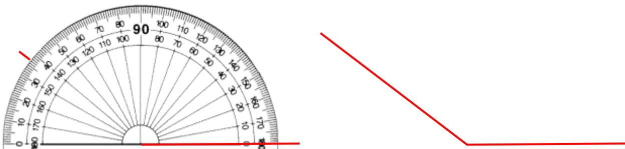
As with measuring, if we have to construct an angle of more than  $180^\circ$ , say  $310^\circ$ , the best way is to subtract the  $310^\circ$  from  $360^\circ$  to get  $50^\circ$  and construct that.
